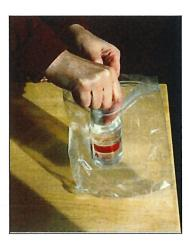
3. The coliform sample bottle may be shipped in a separate coliform sample plastic-foam mailer or with the annual nitrate sample in the large nitrate cooler mailer. Place the zip-close bag with the water sample in the mailer you have available.
