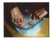
If you are sending the nitrate mailer, place both of the bagged sample bottles into one of the large zip-close bags filled at least three quarters full with ice and then seal. Place the sealed bag in the cooler.
